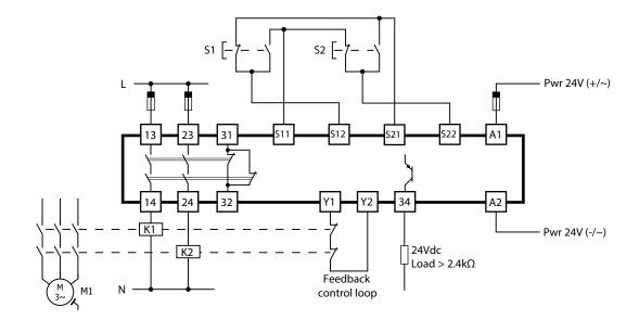
The MS1E41-024 is intended to expand the number of safety outputs of a master safety module. It must be wired correctly to a master safety module to reach the needed safety category.
