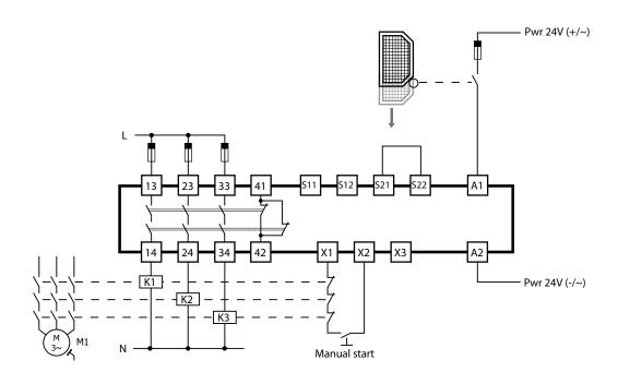
The MS1H21-024 can be used in THCD (Two Hand Control Device) applications up to level III-C according to EN 574 / EN 13851.
