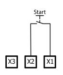
The start button is connected between X1 and X2. The safety inputs S12 and S22 are operated:
