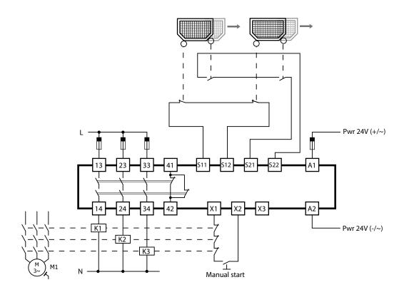
8.5.3 E-gate, safety limit switch and one access monitoring (single channel mode)
