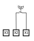
The start button is connected between X1 and X2.
