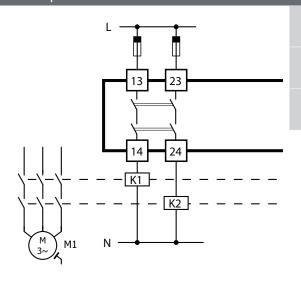
The NO safety outputs switch on (contact closes) when the safety inputs are active and the start/reset is pressed.
