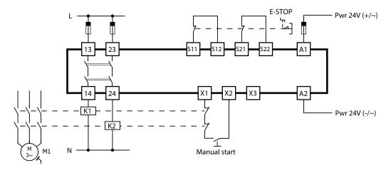
In case of a fault the safety outputs will switch OFF
