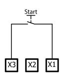
The start button is connected between X1 and X3.
