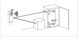
The radio signal generated by transmitter develops with elliptical shape, where receiver and transmitter are located ate the focal points. Because of this the working area shape near the device can condition the operating distance. E.g. the installation in narrow corridors with shielding walls reduces the operating range.
